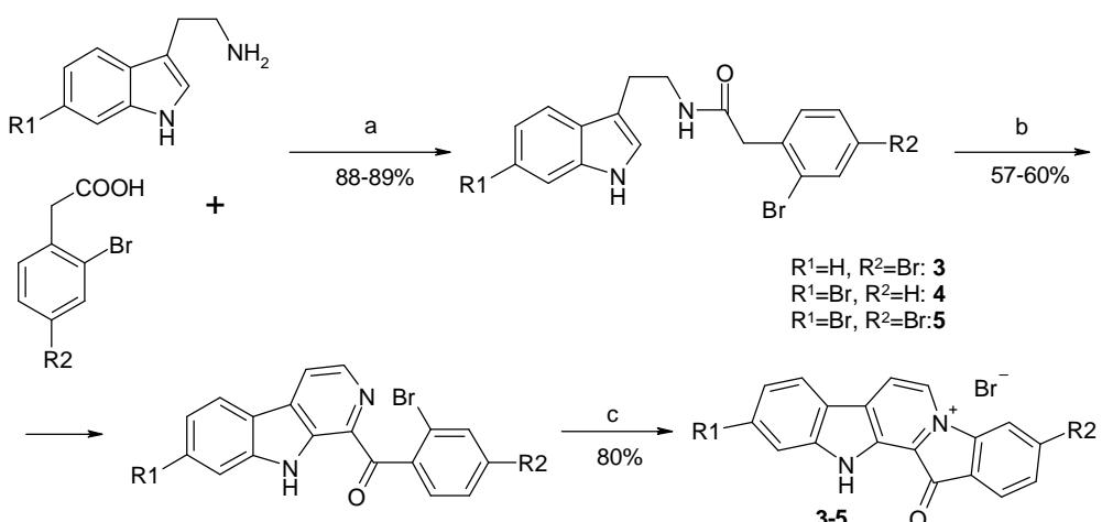
a: DCC, CH<sub>3</sub>CN, reflux, 30 min; b: POCl<sub>3</sub>, CH<sub>3</sub>CN, Ar, reflux, 40 min, then MnO<sub>2</sub>, PhH, reflux, 3 h; c: 220°C, 20 min.
